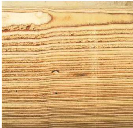
▲ Pic.11 You can see the difference between the roughing and the smoothing cuts. It will always tear out, you just have to make the best cuts to minimise the timber tear out
